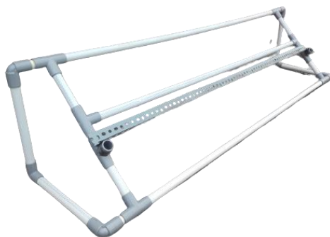
Gambar 1. Rak Paparan Cuaca ( Weathering Rack )
